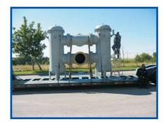
Concord Screen manufactures a full line of manual single basket strainers and duplex body strainers. This style of straining is ideal for both protectionary straining and maintenance of product liquid. Baskets require manual removal and cleaning. The duplex arrangement will allow for uninteruption of system flow. One chamber is isolated for basket removal and cleaning whilst the second chamber remains on line.
